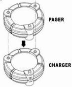
Step4: The pager power LED will go on when the pager is stacked correctly.
